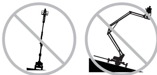
Do not raise the boom unless all four outriggers are lowered, the footpads are in firm contact with the ground and the machine is level.
